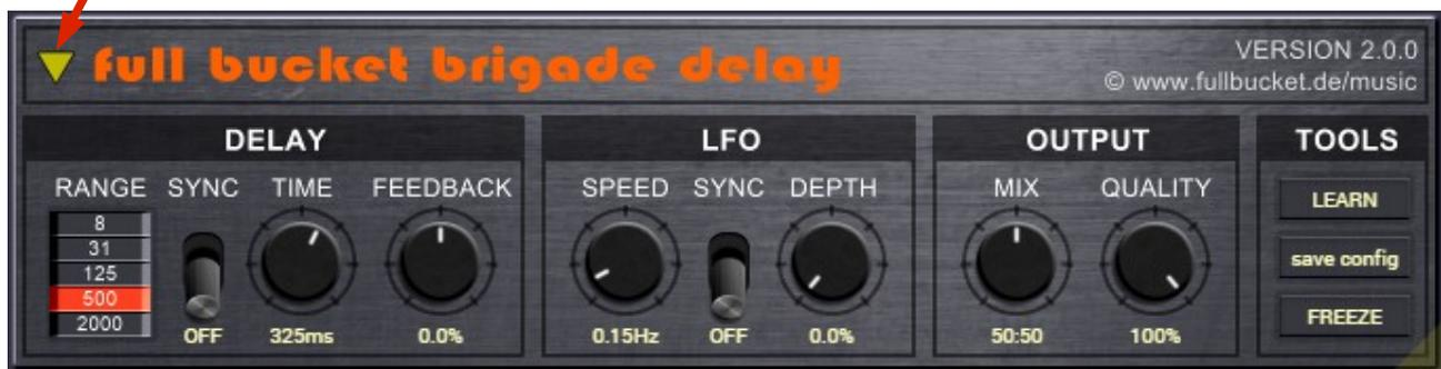
The "LFO" section controls the speed (up to 25Hz) and the depth of the low frequency oscillator modulating the delay time. Here lies the origin of all those nice effects named *Flanger*, *Chorus*, *LSD Trip Echo*, *Psychotic Slapback* etc.
