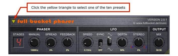
The "LFO" section controls the speed (up to 25Hz) and the depth of the low frequency oscillator modulating the Phaser frequency. The mix between original and effect is set in the "OUTPUT" section.
