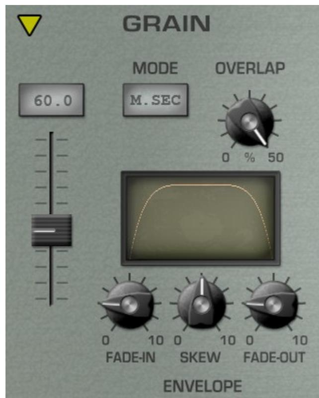
The OVERLAP control allows the separate grains to overlap by up to 50%. Especially in FREQ and MIDI mode this is useful to avoid harsh discontinuities at grain boundaries.
