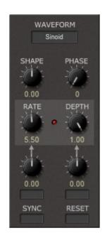
The LFO module has two modulation outputs: LFO (bipolar) and LFO+ (unipolar).
