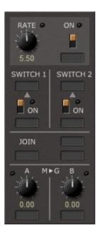
The Sequencer Clock module has six gate/trigger outputs (Clock, Switch 1, Switch 2, Join, M2G A, M2G B).
