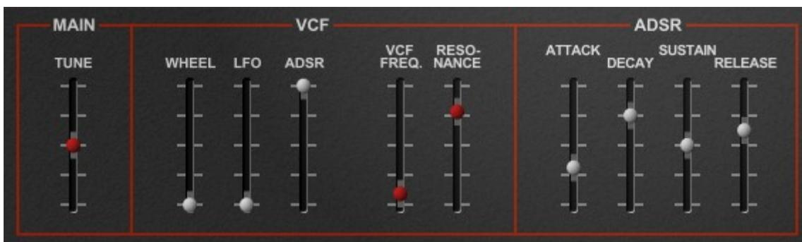
In the subsection "MAIN", the slider "TUNE" controls the master tune of the instrument. Note that this refers to all three sections *Synthesizer*, *String*, and *Synth Bass*.
