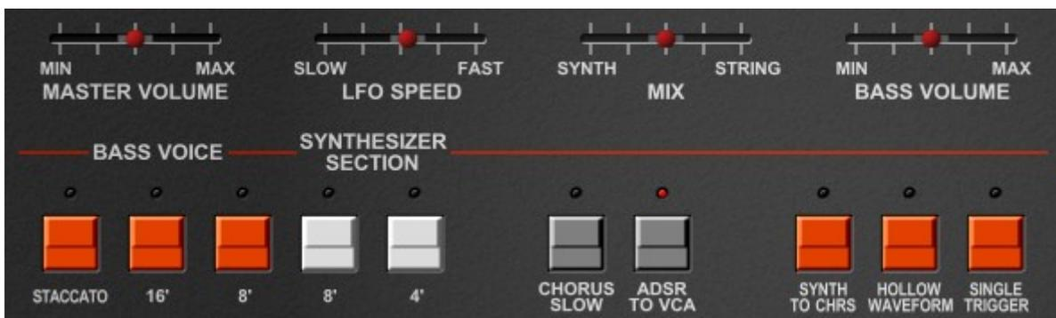
The *Synthesizer's* VCF and ADSR are explained later. The *Synth Bass* section's 2-pole VCF and its envelopes are set to fixed values – the only thing you can modify here is the decay to a shorter time via the "STACCATO" switch. Once a *Synth Bass* preset is selected, the *Synth Bass* only plays notes below or equal G2 (MIDI note #55) while the *Synthesizer* only plays notes above G2.
