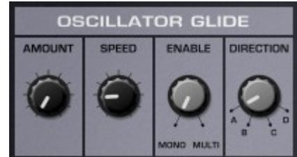
Note that modes B and C will have no effect when SYNC is on! Why? Because Oscillator 2 is clocked by Oscillator 1 then. No “Hello Again”<sup>3</sup>... ☹
