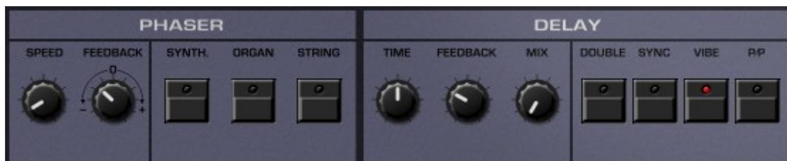
The Phaser is loosely based on the famous Electro Harmonix *Small Stone* with its 4-stage allpass filter design. SPEED sets the modulation rate and FEEDBACK the positive or negative feedback level – extreme settings can make your ears tingle. The Phaser works in stereo and can be activated for each of the three sound sections individually.
