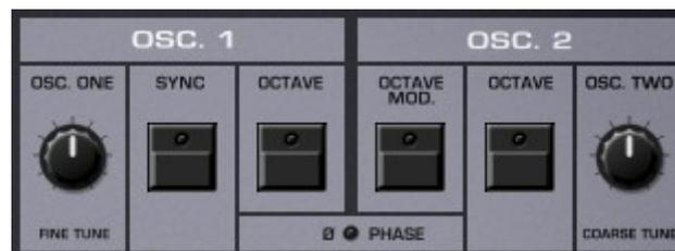
Oscillator 1 can be tuned by  $\pm 1$  semitone and Oscillator 2 by  $\pm 7$  semitones. The "Beating" that results from oscillator detuning is visualized via the PHASE LED.
