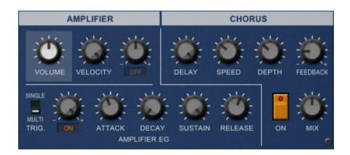
Finally the signal is processed by a wide-range stereo Chorus unit (which also can be deactivated). The Chorus has controls for effect mix, manual delay time, modulation depth and speed, and positive or negative feedback.
