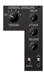
The polarity switch changes the output polarity of the GEG. Note that in the upper ("positive") position the output will range from -5 to 0 (virtual) Volts while in the lower ("negative") position from 0 to +5 Volts. This may seem a bit odd but that's what it is on the original PS-3100 too.
