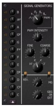
An interesting feature is the *micro-tuning* option. Each of the 12 keys can be tuned individually, allowing for other (not necessarily well-tempered) tunings like *Pythagorean* or *Wendy Carlos' Super Just* tuning etc. The small button at the bottom of the tuning knobs opens a menu with 14 predefined micro-tuning templates. Here it is also possible to load and/or save the tuning settings from/to a Scala (\*.scl) file.
