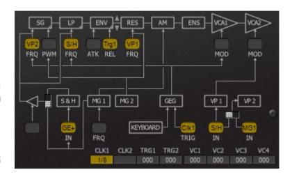
Strictly speaking there are two types of sources and targets: *modulations* and *triggers*. For example the "ATK" target of the EM continuously modulates the Attack time while the "REL" target waits for a trigger signal to release the envelopes.
