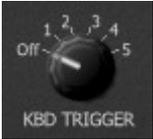
The GEG can be triggered by any trigger signal patched into one of the two plugs *TRG1* and *TRG2*. Of special interest is the "KBD TRIGGER" source: Here you can select how many keys (1 to 5) have to be pressed before this trigger source is triggered (in the "Off" position the keyboard by default does not trigger at all).
