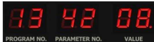
To change the value of a parameter you have to use the *DOWN* and *UP* buttons. If the value of the parameter has changed, the display will show a dot at *VALUE*. Note that this only applies as long as you do not select a different parameter or program (this is a funny feature of the original *Poly-800* transported into the 21<sup>st</sup> century).
