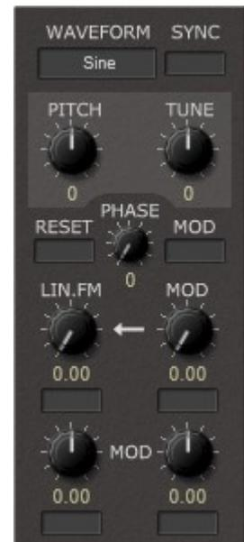
The *Linear FM Oscillator* module has one audio and one *Sync* output.
