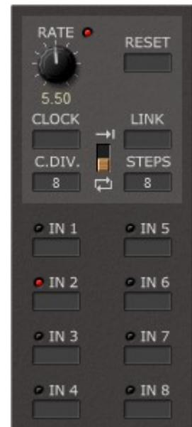
The *Sequential Switch* module has one modulation output and fourteen trigger outputs: *Clock*, *Clock Div*, *Clock Link* (clocks only in non-looping mode when the sequencer has finished the last sequence step), *Reset* (clocks when the sequencer resets to step 1), *Stop*, *Step Active* (clocks each time a step with active modulation input is reached), *Step 1–8* (clocks for each individual step).
