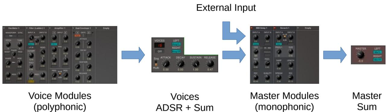
The voice signals generated by the Voice modules are shaped by individual ADSR envelope generators and then summed up to form the *Voices Sum* stereo signal. This signal along with an external input signal can be used to feed the Master modules. The final output can then be selected from the output of a Master module (if applicable) or the *Voices Sum* signal.
