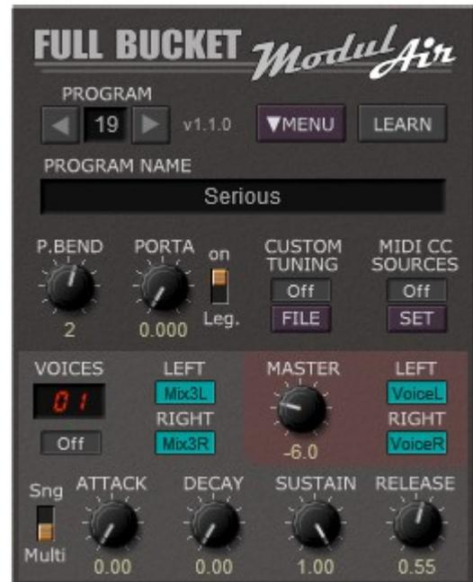
The volume envelope of a voice signal is shaped by an ADSR generator with adjustable trigger mode (*Single* or *Multiple*). Thus, you do not have to add extra Amplifier and Envelope modules (although you can) for your sound patch. If you turn *Release* to the very right (i.e. to 1.00), the ADSR goes into *HOLD* mode. Note that this may have a heavy impact on CPU performance!
