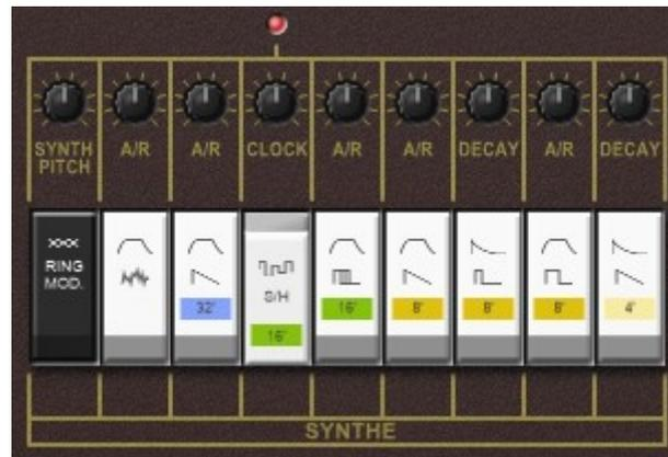
There is also an additional *Ring Modulator* switch that replaces the standard output of the *Synthe* section with the Ring-modulated signal of the *Synthe* and the *Instrument* sections. Note that in order to hear any sound when *Ring Mod* is on, at least one preset of both sections has to be activated.
