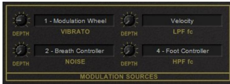
There are four modulation paths available for the *Stigma*: *Vibrato* (Joystick 1 Y axis up; controls the Vibrato modulation depth), *Noise* (Joystick 1 Y axis down; controls the Noise modulation depth), *LPF fc* (Joystick 2 X axis; controls the cutoff of the *Synthe* lowpass filters), and finally *HPF fc* (Joystick 2 Y axis; controls the cutoff of the *Synthe* highpass filter).
