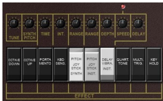
Pitch bending and modulation by *Vibrato* or *Noise* (see section *From Joystick To Wheels: Modulation Sources*) can be activated separately for the *Synthe* (VCO 2) and *Instrument* (VCO 1) sections via the *Pitch Joystick* switches; the *Range* knobs control the amount of the modulation effect respectively. The *Delay Vibrato* only applies to the *Instrument* section. Knobs are available for *Vibrato* depth, speed, and delay time.
