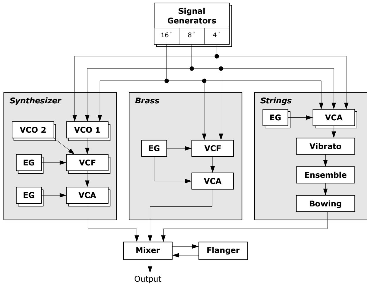
Note that while the *Synthesizer* section is truly polyphonic (one VCO 1, VCO 2, VCF and VCA per voice), the *Brass* section is *paraphonic*: There is only one VCF and one VCA for all voices.
