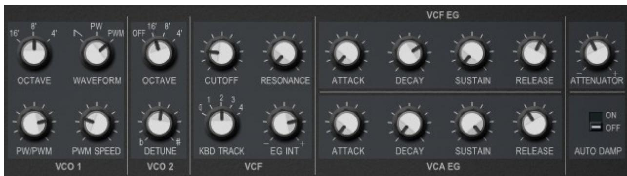
VCO 1 offers three waveforms: *Sawtooth*, *Pulse Width* and *Pulse Width Modulation*, where the latter is modulated by a dedicated LFO (Low Frequency Oscillator). VCO 2 only produces a Sawtooth wave and can optionally be turned off.
